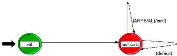
Figure 6 The Process Model of Multicast Generator
