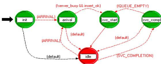
Figure 7 The Process Model of Input Queue
