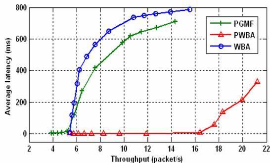
Figure 10 Graph of average cell latency as a function of throughput
