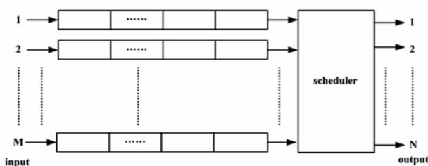
Figure 1 The multicast scheduling model based on input-queued switch
