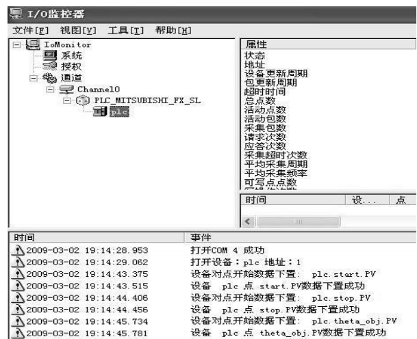
Figure 5 the experiment result of RS485 serial communication through high-speed data communication card
