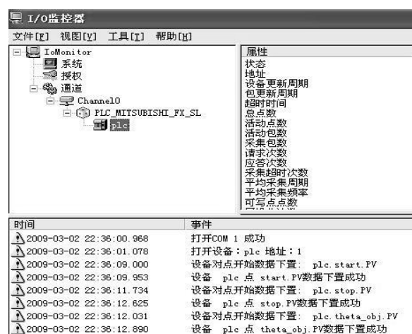
Figure 4 the experiment result of RS232 serial communication through programmable port
