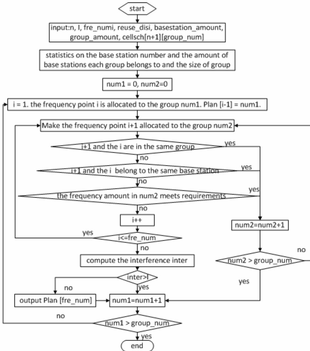
Figure 1. Flow chart of the algorithm about channel allocation
