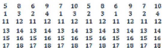
Frequency points 5, 8, 6, 9, 7 and 10 are fixed, allocated to the type 1 and 1, 3, 2 and 4 are also fixed, allocated to the type 2. Points 11, 12, 13, 14, 15, 16, 17 and 18 are dynamic, used in turn with the train mobile.
