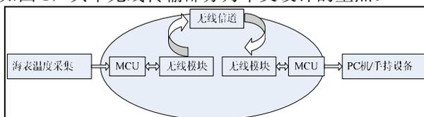
Figure 1. Diagram of sea surface temperature collection system
