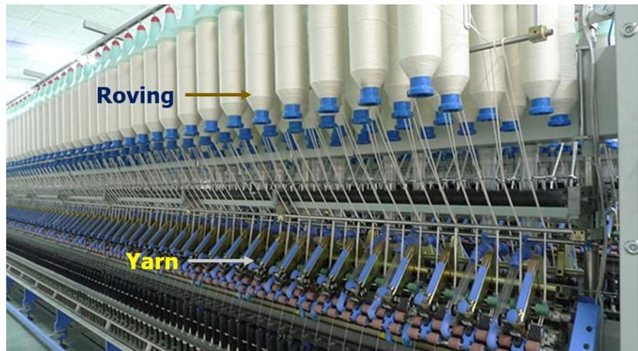
**Figure 1.** Ring frame producing yarn from roving.
