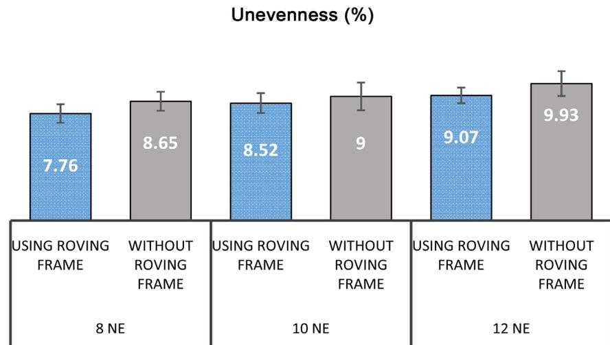
**Figure 3.** Influence of roving frame on Unevenness (%).
