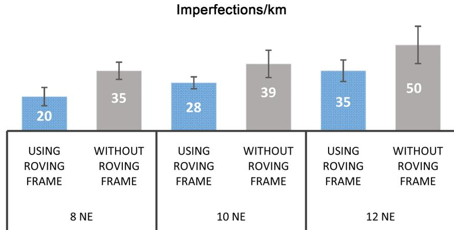
**Figure 4.** Influence of roving frame on IPI.
