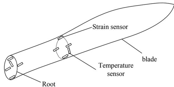
Figure 2 Strain sensor configuration in wind turbine blade
