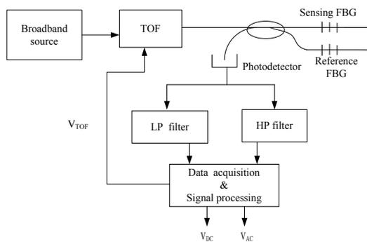
Figure 1 FBG sensor system
