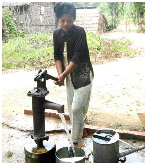
Figure 14. Tubs wells with hand pump used in Mekong Delta.
