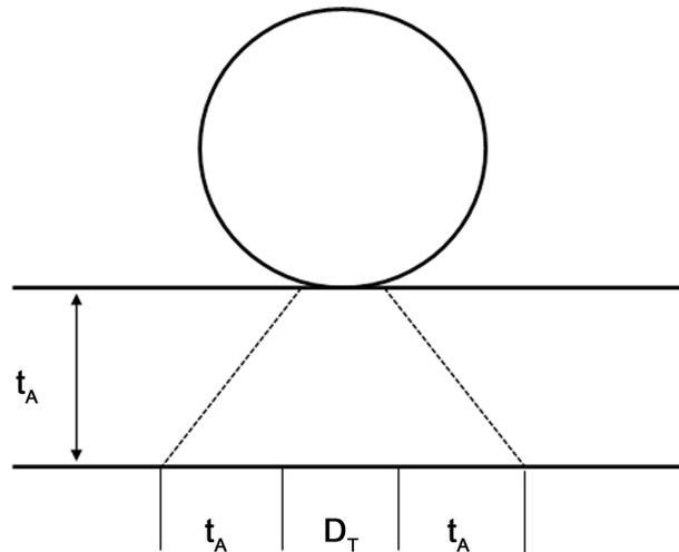
**Figure 4.** Stress distribution diagram.  $t_A$  is the Asphalt thickness.  $D_T$  is the tire footprint diameter thickness.
