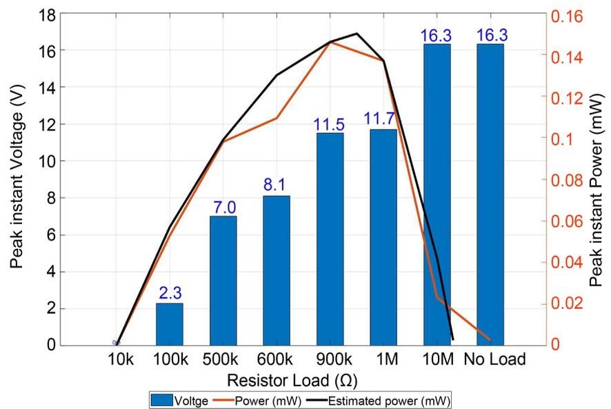
**Figure 12.** Instantaneous peak voltage and power for varying resistor loads (asphalt test).
