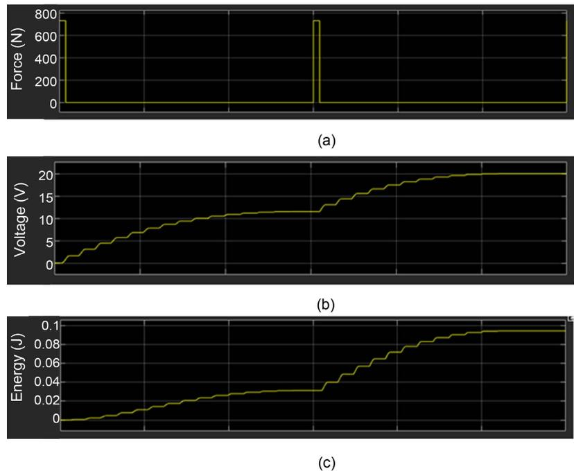
**Figure 6.** SIMULINK Results 3 layers, 5 mm thickness using one care passing that stresses the piezoelectric module using the front and the back tires. (a) Force per Stack (N); (b) Storage Capacitor Voltage (V); (c) Storage Capacitor Energy (J).
