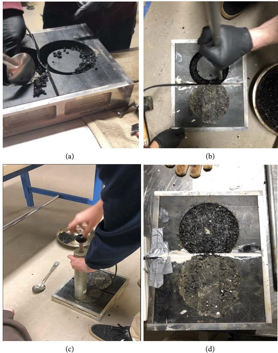
**Figure 10.** (a) Layering Aquaphalt on top of RPEH; (b) Compacting Aquaphalt; (c) Tamping surface Aquaphalt layer; (d) RPEH embedded under Aquaphalt.
