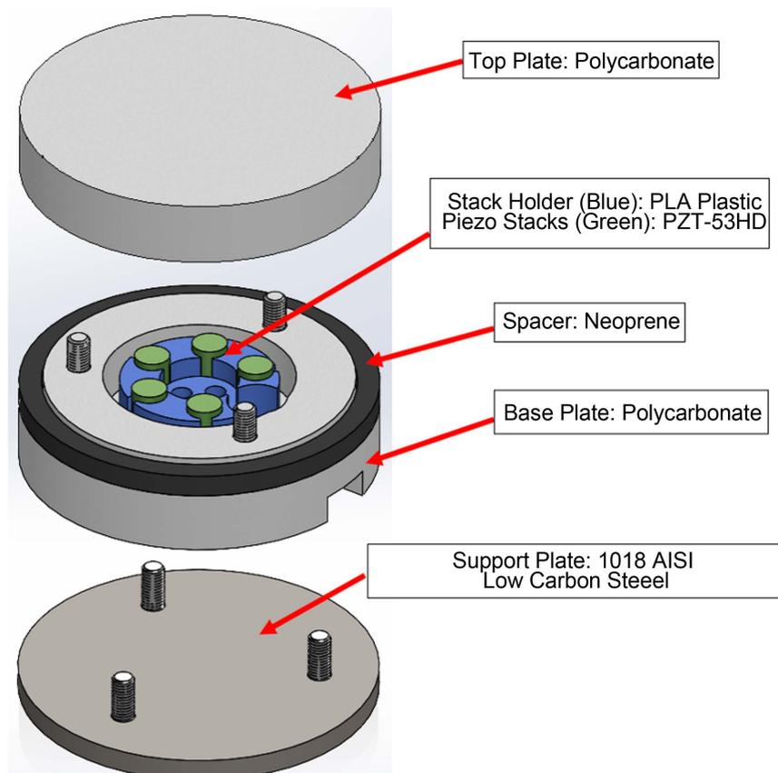
**Figure 2.** Expanded view of harvester module with part name and material identified.
