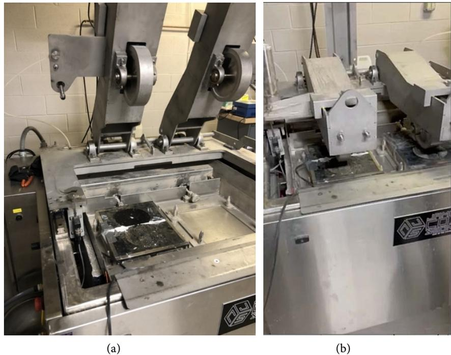
**Figure 11.** (a) RPEH in Hamburg wheel tracker; (b) Hamburg wheel tracker running.
