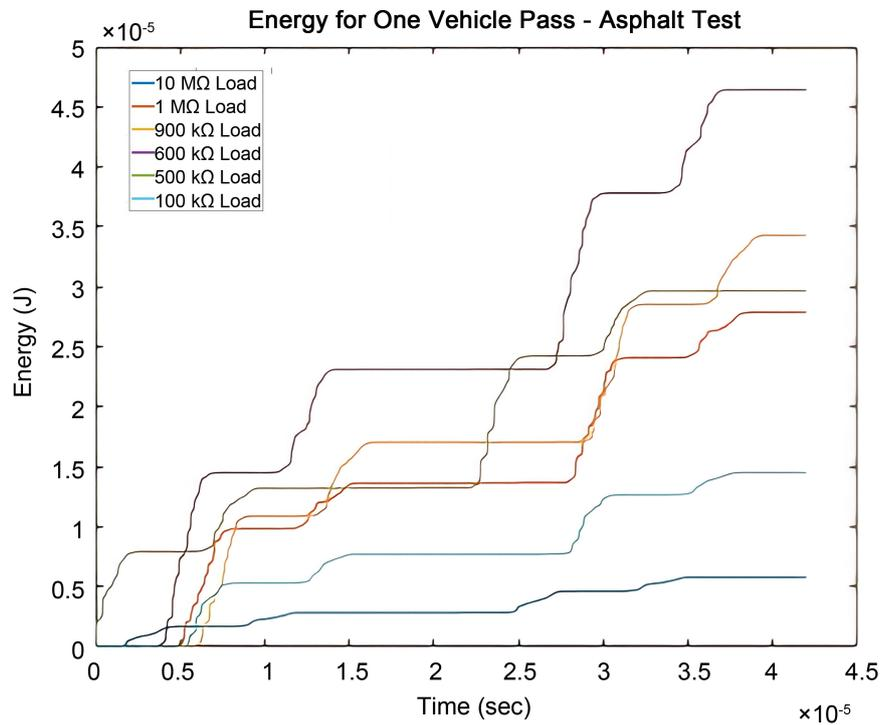
**Figure 13.** Transient energy for one vehicle pass-asphalt test.
