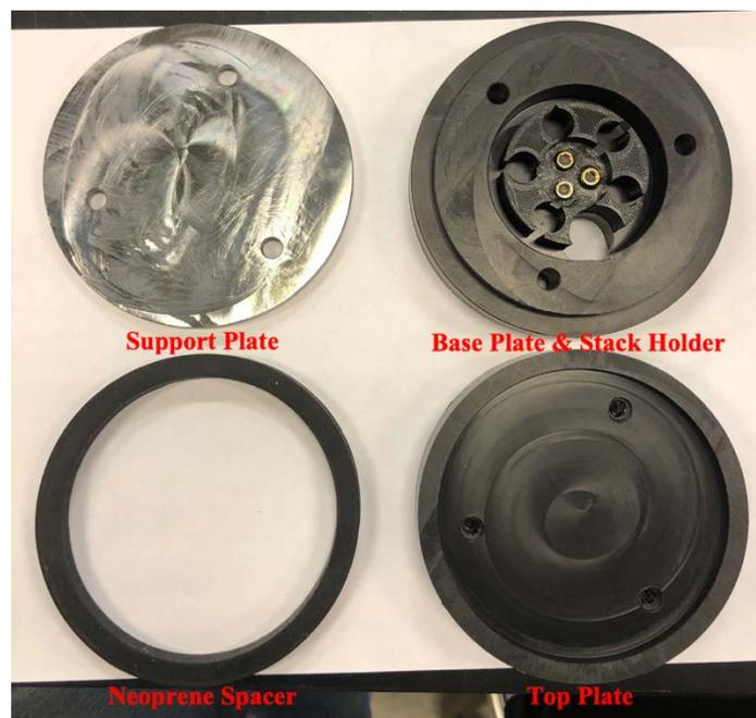
**Figure 8.** Disassembled RPEH with labeled parts.
