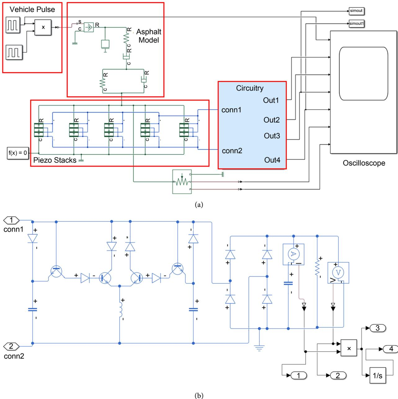
**Figure 5.** SIMULINK RPEH block diagram. (a): Block diagram; (b) SIMULINK SSHI rectifier circuit (circuitry block in (a)).
