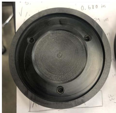
**Figure 9.** Top plate with added clearance.
