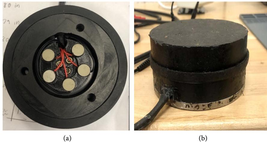
**Figure 7.** Completed RPEH prototype. (a) The five stacks installed in RPEH; (b) Assembled RPEH.
