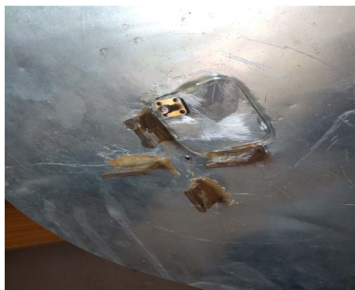
Figure 14. SMA connector attached to the backside of the reflector.
