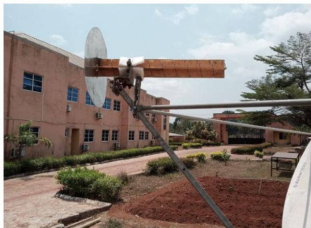
Figure 19. Fabricated Antenna mounted as feed on a 2.4 metre off-set Parabolic Dish at the Observatory Complex of the Centre for Basic Space Science, Nsukka.
