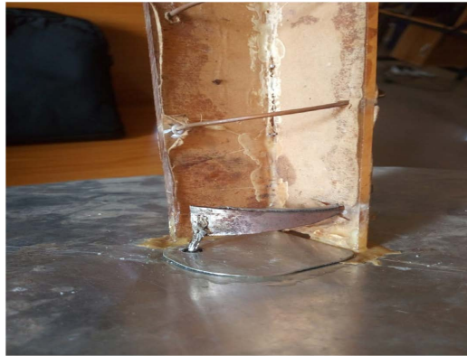
Figure 13. Showing SMA connector inner pin soldered to the triangular metal strip impedance matching structure.
