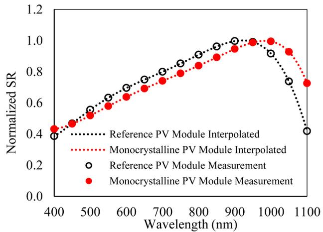
Figure 14. Spectral responsivity of monocrystalline PV module.
