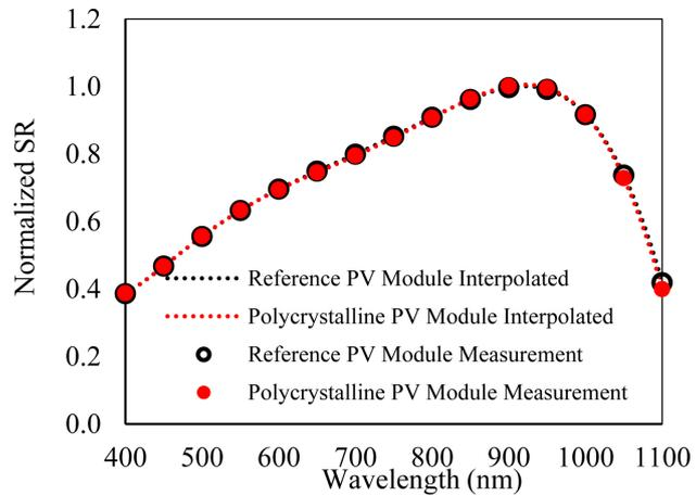
Figure 13. Spectral responsivity of polycrystalline PV module.
