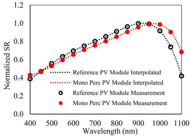
Figure 16. Spectral responsivity of MonoPerc PV module.
