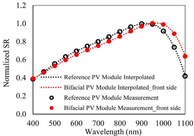
Figure 15. Spectral responsivity of bifacial PV module.
