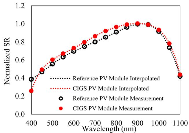
Figure 18. Spectral responsivity of CIGS\_2 PV module.
