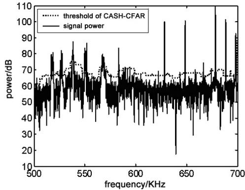
Figure 6. Threshold by CASH-CFAR
