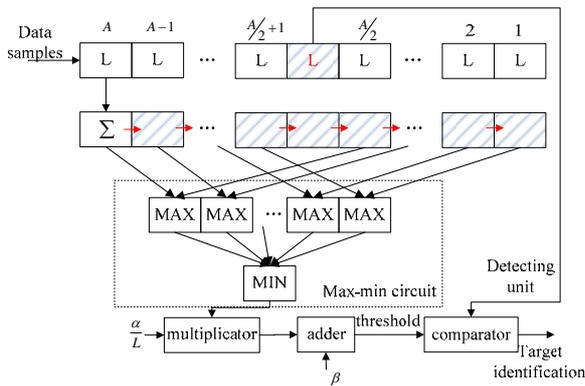
Figure 2. Principle of the modified CASH-CFAR circuit
