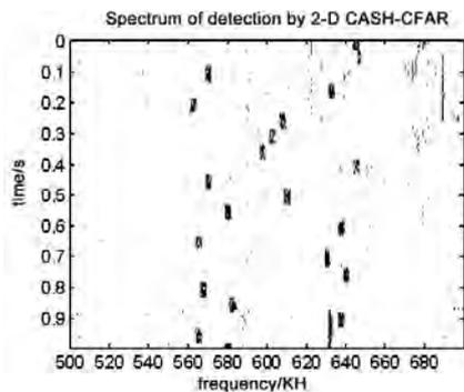
Figure 8: Identification of 2-D MCASH-CFAR
