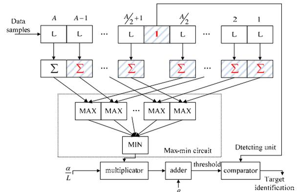
Figure 1: Principle of the CASH-CFAR circuit
