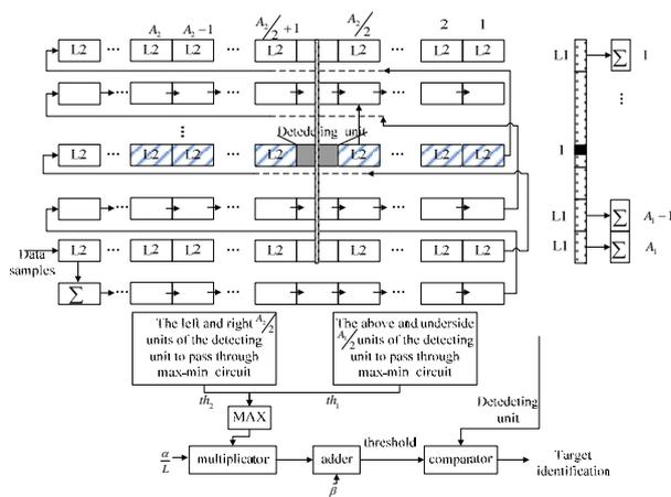
Figure 5. Principle of 2-D MCASH-CFAR circuit
