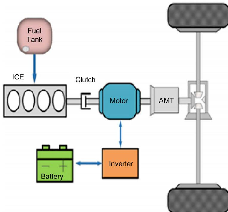
Figure 6. Powertrain configuration host vehicle.
