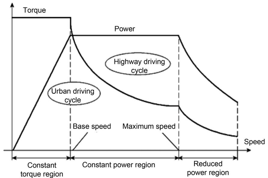
**Figure 8.** Typical speed-torque characteristics of EV & HEV from electric traction motor.
