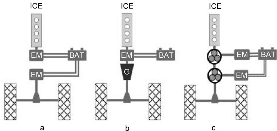
**Figure 1.** Configurations of hybrid powertrains.
