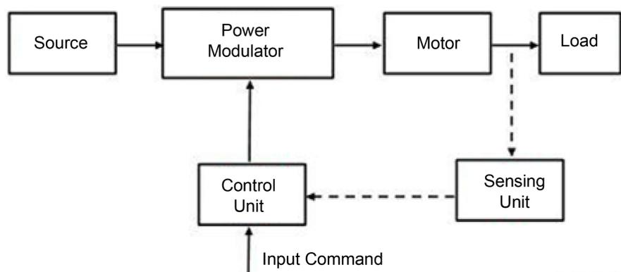
**Figure 7.** Block diagram of the electrical drive.
