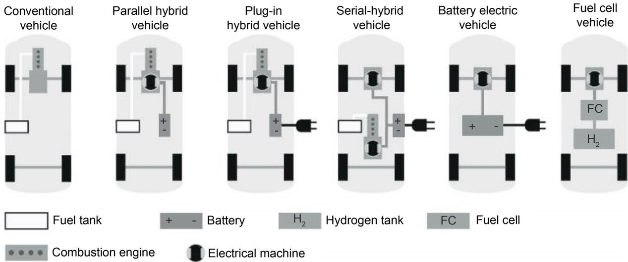
**Figure 4.** Electric propulsion system diversity vs. conventional propulsion.
