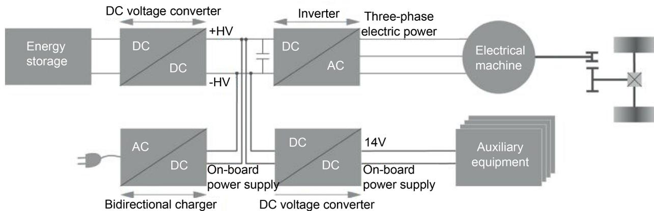
**Figure 3.** Electric drivetrain architecture.
