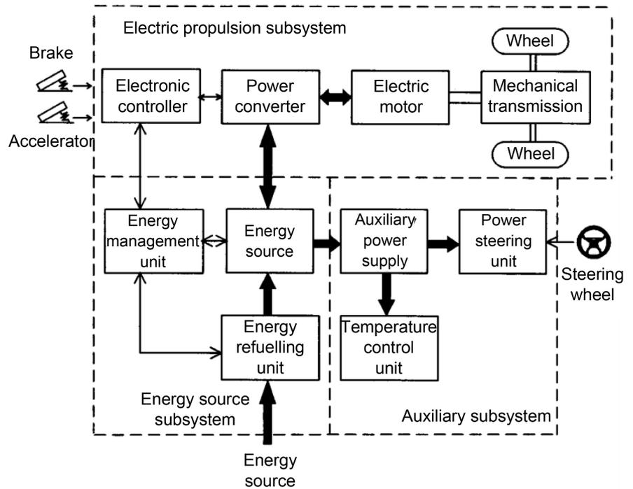
Figure 5. Electric vehicle composition.
