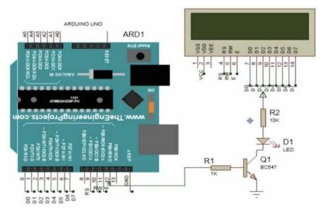
Figure 5. Li-Fi transmitter block.
