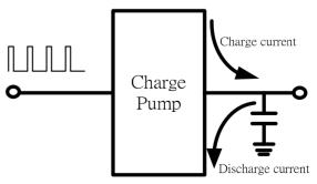
Figure 6. Charge and discharge current.
