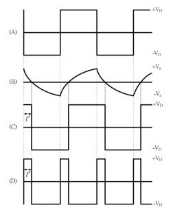
Figure 4. (A) Reference clock (B) The output of the STC circuit (C) The output of the voltage comparator (D) The output of the PD.
