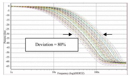
Figure 9. The 3-dB frequency variation in sixty corners (without tuning).
