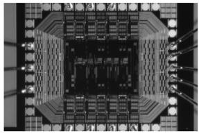
Figure 11. Die photo of the proposed circuit.
