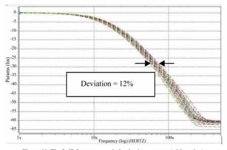
Figure 10. The 3-dB frequency variation in sixty corners (with tuning).
