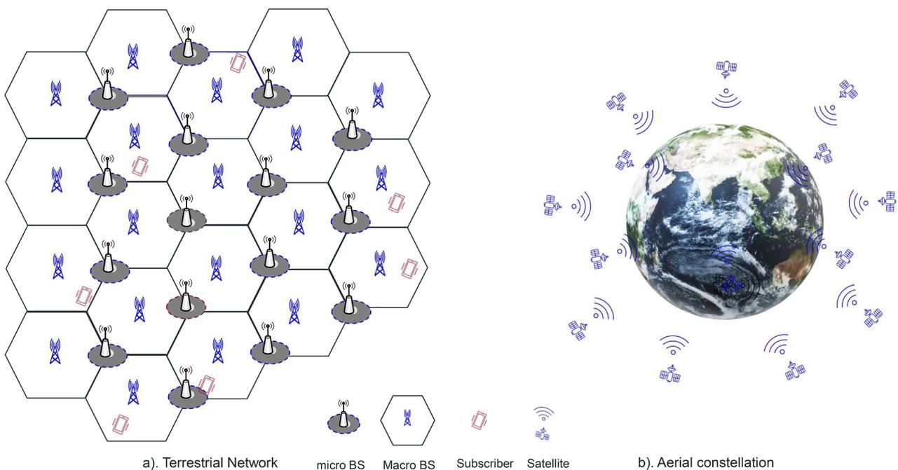
**Figure 2.** Terrestrial network and satellite constellations.
