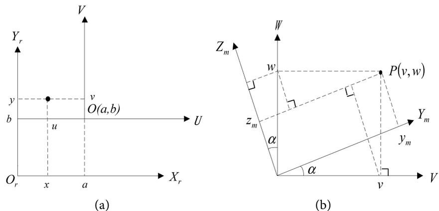
**Figure 3.** Schematic diagram of translation and rotation of coordinate systems. (a) Translation; (b) Rotation.
