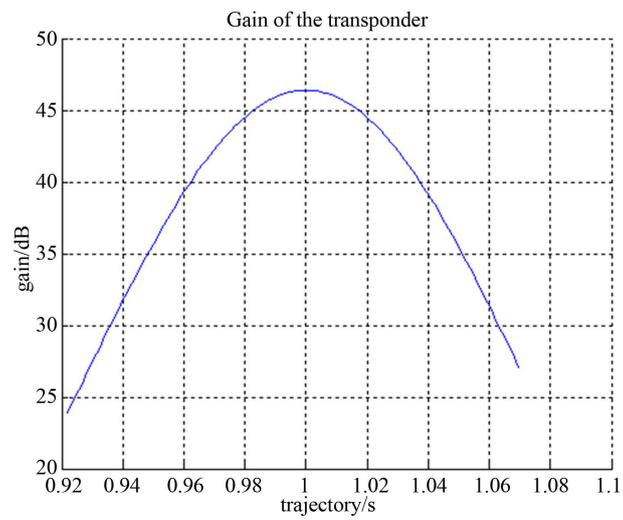
**Figure 10.** Gain change of transponder in measuring segment.
