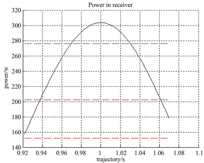
**Figure 11.** Received power of exterior trajectory measurement equipment in measuring segment.
