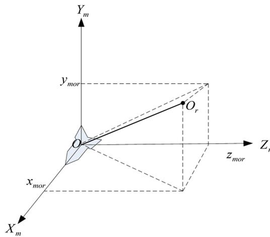
**Figure 1.** Schematic diagram of body coordinate system.
