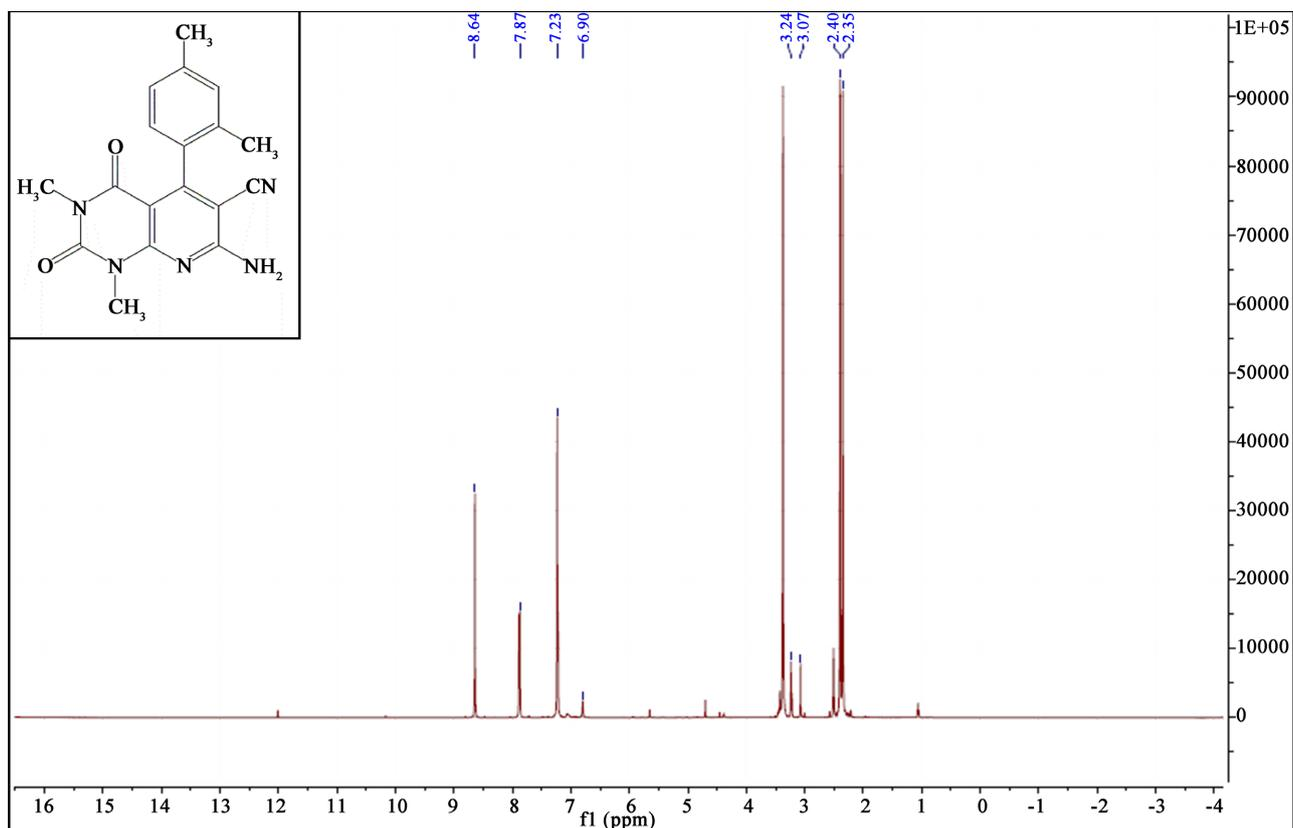
Figure 8.  $^1\text{H}$  NMR spectrum of 4f.
