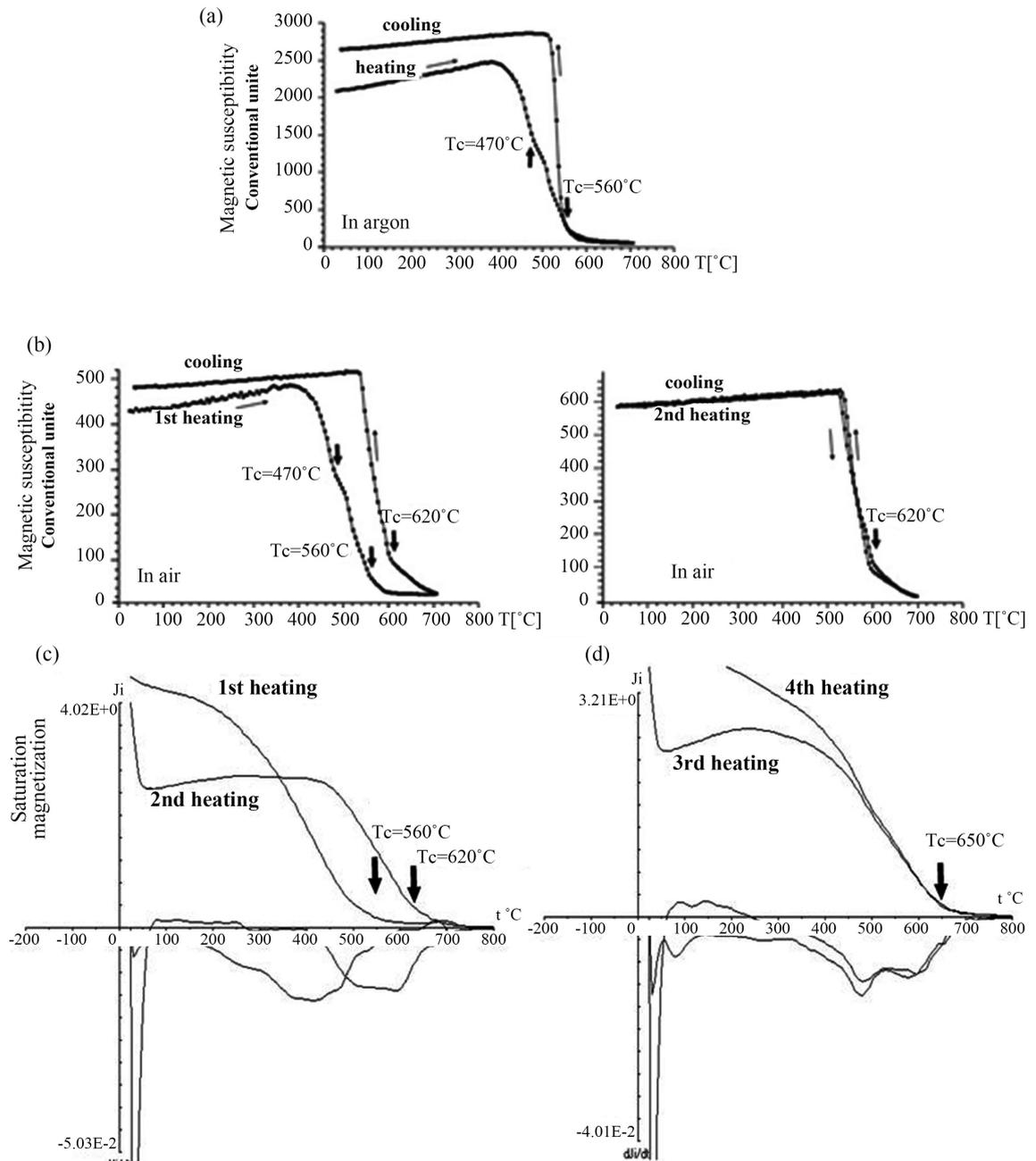
**Figure 7.** Magnetic properties of the Ilekt sample: (a)-(b) thermocappametry curves in argon (a) and air (b); (c) dependence of saturation magnetization on temperature (the lower part of the graphs are differential curves).
