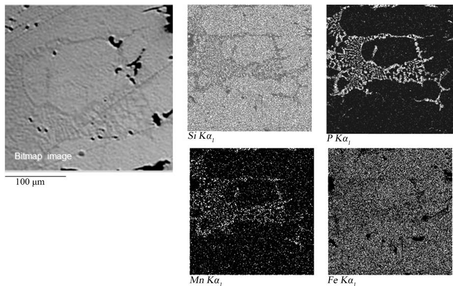
**Figure 6.** Distribution of mineral phases in characteristic X-ray radiation.
