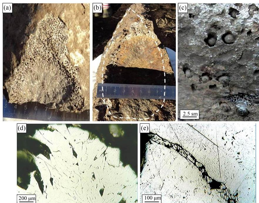
**Figure 4.** Features of the morphology of the gupeite body: (a)-(b) wedge-shaped cross-section of the “Ilekta” sample on the chip (photo of one of the hunters, Gennady Porfirievich.Berzin); (c) bubble surface; plastic (d) and brittle (e) deformations clearly visible on the slice.
