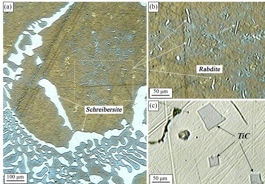
**Figure 5.** Mineral phases of “Ilecta” in reflected light: (a)-(b) eutectic decomposition of gupeite with schreibersite and needle crystals of rhabdite in gupeite (structural etching of HCl); (c) crystals of Ti carbide in gupeite.
