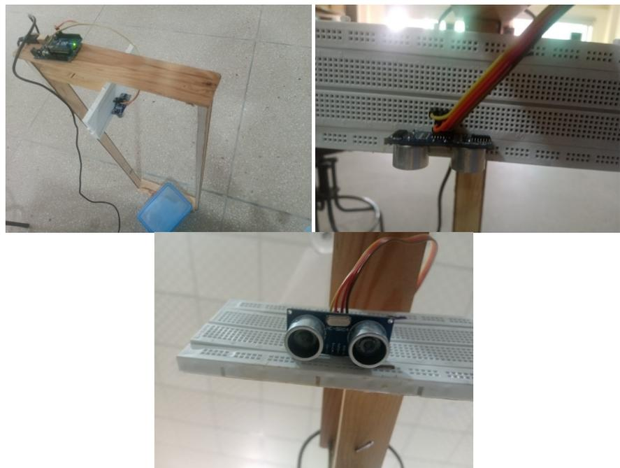
**Figure 1.** Experimental setup for the determination of acceleration due to gravity during free fall motion.
