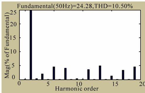
**Figure 9.** FFT analysis of the supply current after APF input based on adaptive interference canceling theory
