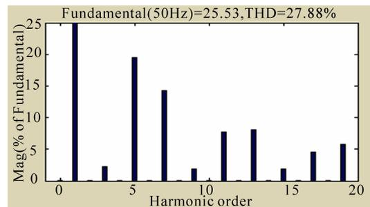
Figure 8. FFT analysis of the supply current before APF input
