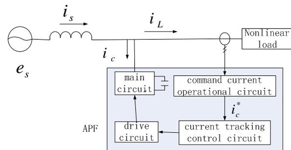
Figure 1. Basic principle block diagram of an active filter
