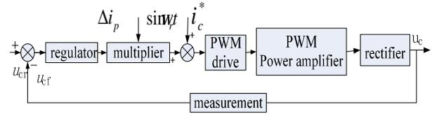
Figure 4. DC voltage control block diagram
