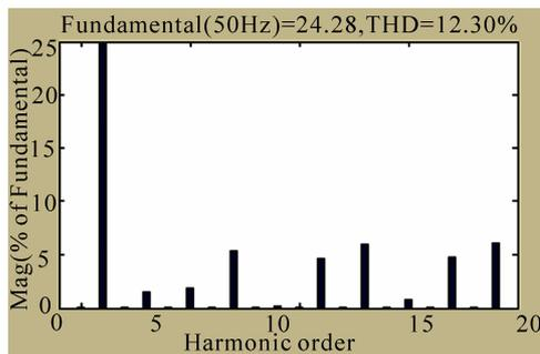
**Figure 10.** FFT analysis of the supply current after APF input based on instantaneous inactive power theory
