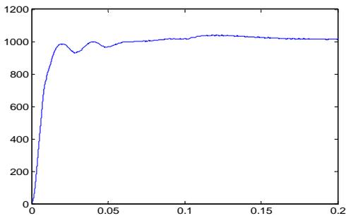
Figure 7. DC side capacitor voltage of active filter
