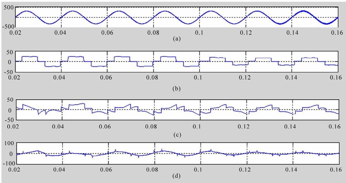
Figure 6. Simulation result of detection for harmonic and reactive currents. (a) ac source voltage for phase A, (b) power supply currents for phase A before filter input, (c) harmonic and reactive reference current from adaptive detection, (d) power supply currents for phase A after filter input
