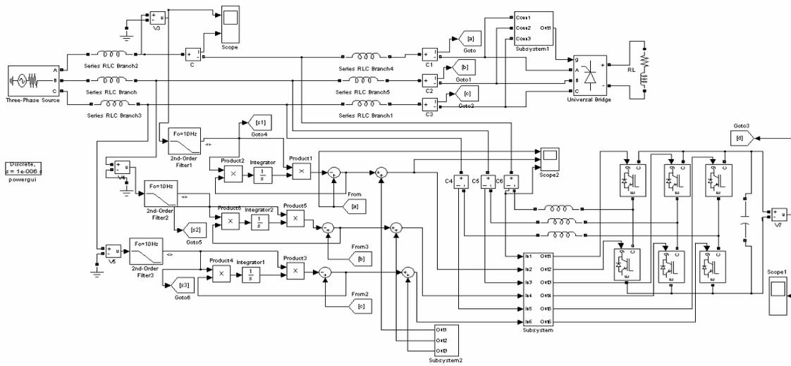
Figure 5. Active filter simulation model
