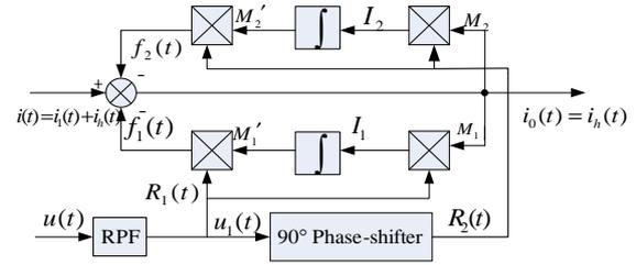
Figure 3. Adaptive detecting diagram for harmonic currents
