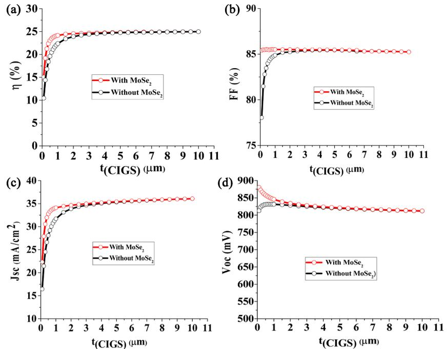
**Figure 4.** Effects of absorber layer thickness on cell performance for cell with and without  $\text{MoSe}_2$  layer (30 nm thick). (a) conversion efficiency  $\eta$ , (b) fill factor  $FF$ , (c) open circuit voltage  $V_{oc}$  and (d) short circuit current  $J_{sc}$ .
