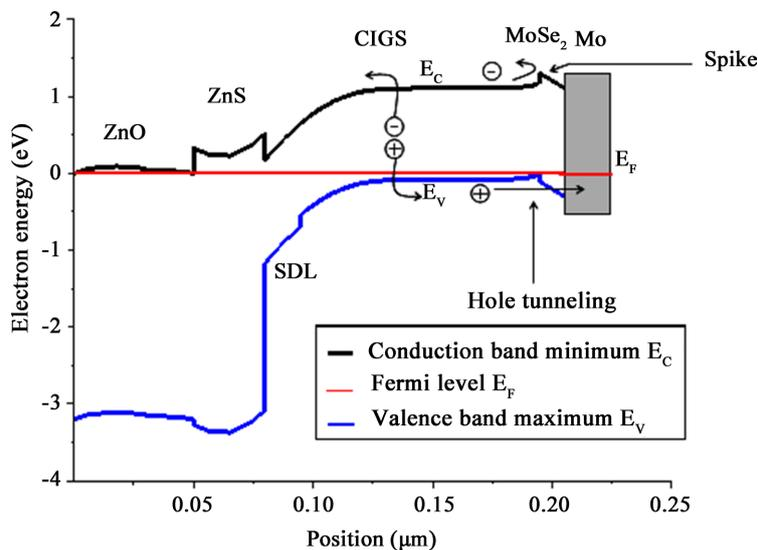
**Figure 5.** Calculated band structure of the CIGS solar cell with additional MoSe<sub>2</sub> layer under zero-bias voltage.
