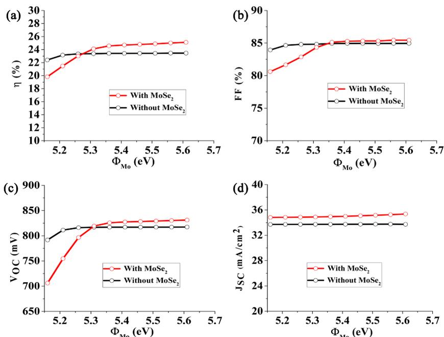
**Figure 6.** Effects of the Schottky barrier height on cell performance for MoSe<sub>2</sub>-free cell and cell with additional MoSe<sub>2</sub> layer. (a) conversion efficiency  $\eta$ , (b) fill factor FF, (c) open circuit volatge  $V_{\text{OC}}$  and (d) short circuit current  $J_{\text{SC}}$  (absorbing layer thickness is 1.5  $\mu\text{m}$ ).
