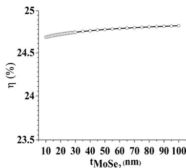
**Figure 2.** Effect of the MoSe<sub>2</sub> layer thickness on the cell efficiency (absorbing layer thickness is of 3  $\mu\text{m}$ ).
