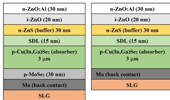
Figure 1. Schematic configuration of the optimized CIGS-based solar cell (a) with and (b) without MoSe<sub>2</sub> layer.
