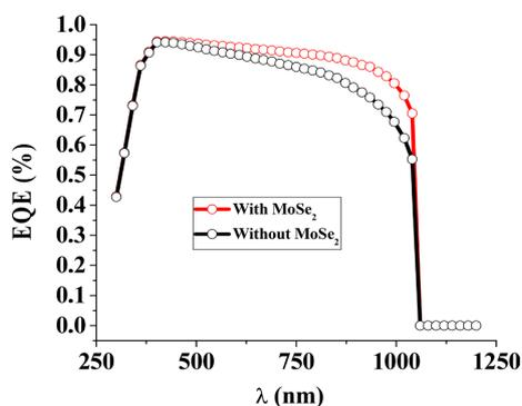
**Figure 3.** Effect of MoSe<sub>2</sub> layer (30 nm thick) on the EQE (absorber thickness is of 1.5  $\mu\text{m}$ ).
