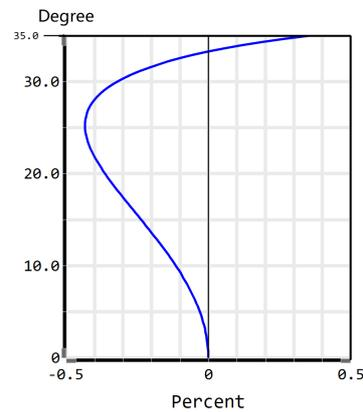
**Figure 4.**  $f$ -theta distortion of the optimized wide-angle lens group.
