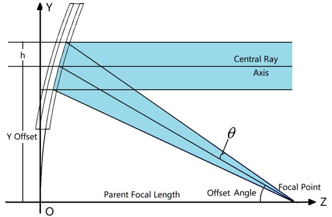
Figure 2. Diagram of off-axis parabolic mirror.
