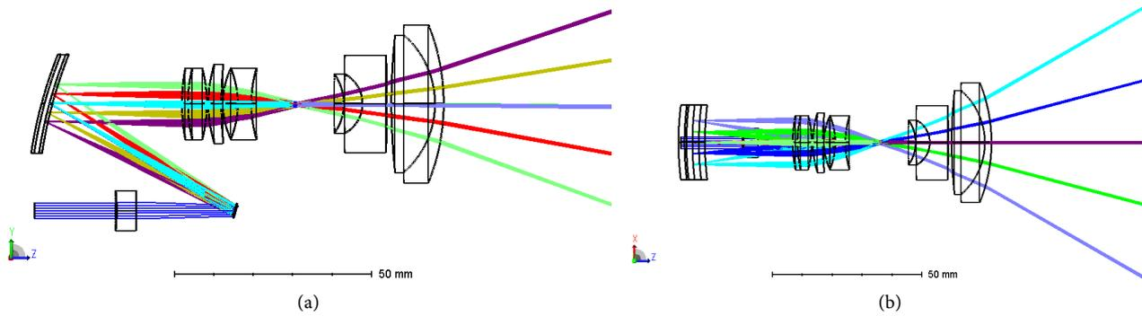
**Figure 1.** The scheme of the scanning system. (a) Front view of the system; (b) Top view of the system.
