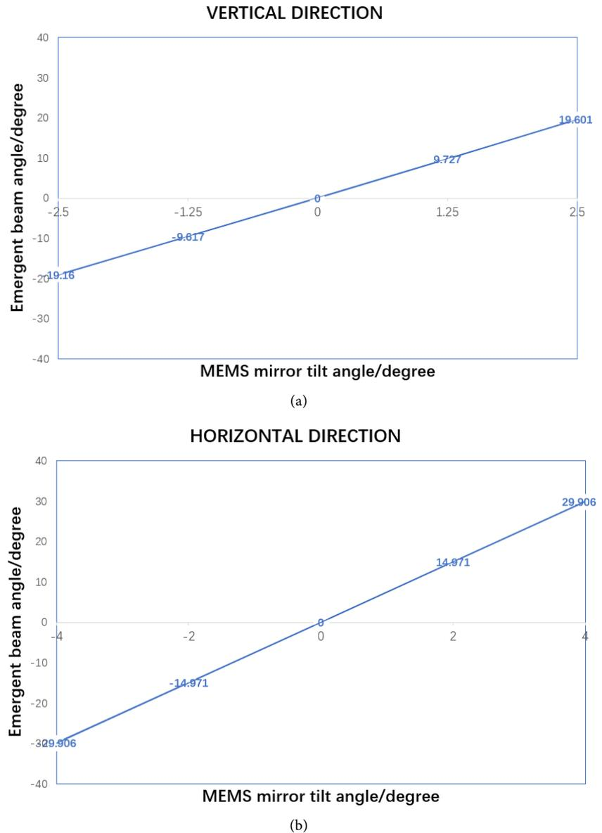
**Figure 5.** The relationships between tilt angles and emergent angles. (a): vertical direction (b): horizontal direction.
