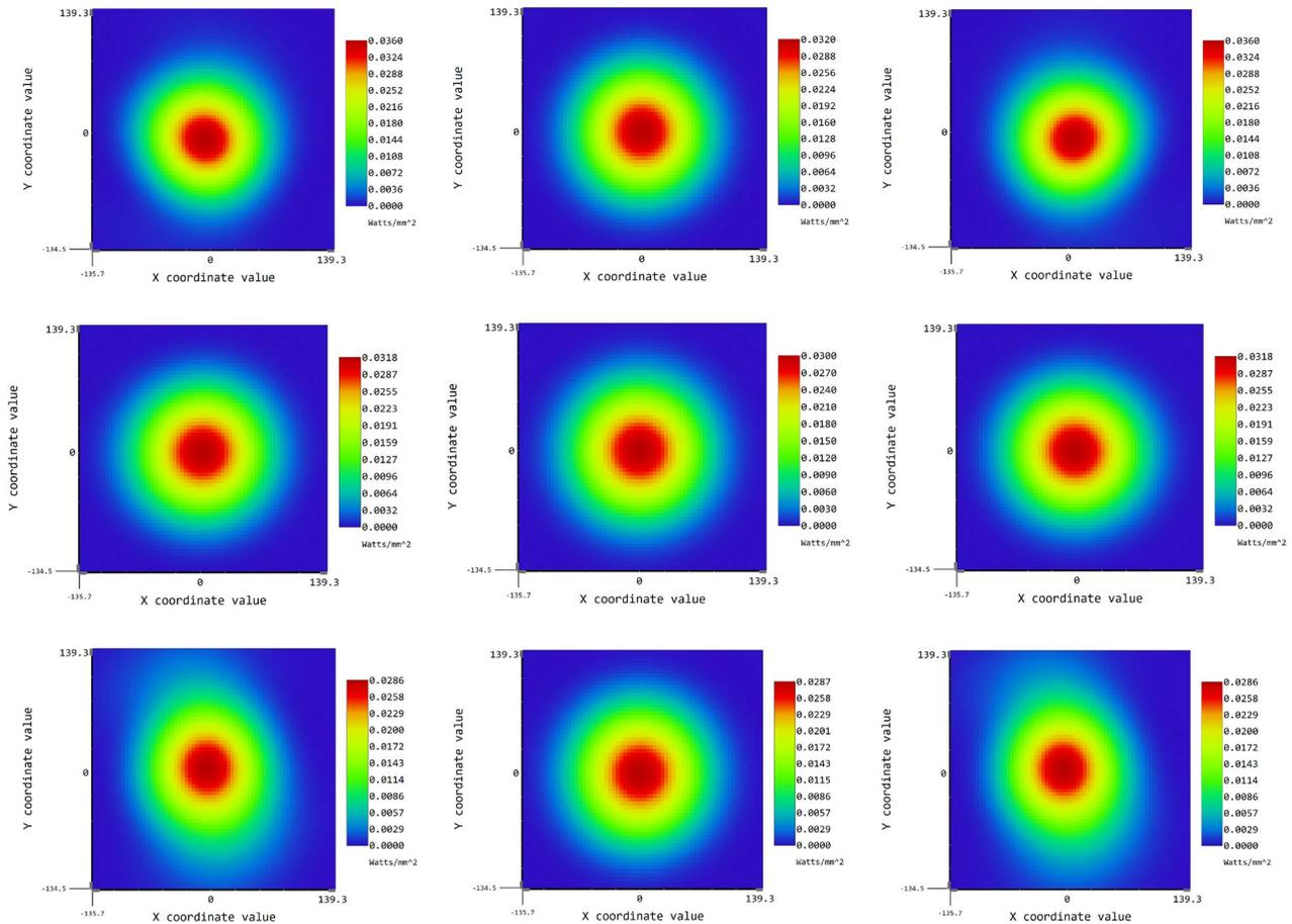
**Figure 6.** Beam spot patterns with different MEMS mirror tilt angle at a distance of 100 m away. The scale is 275 mm. The three line from the upper left to lower right are the cases corresponding the tilt angles  $(2.5^\circ, -4^\circ)$ ,  $(2.5^\circ, 0^\circ)$ ,  $(2.5^\circ, 4^\circ)$ ,  $(0^\circ, -4^\circ)$ ,  $(0^\circ, 0^\circ)$ ,  $(0^\circ, 4^\circ)$ ,  $(-2.5^\circ, -4^\circ)$ ,  $(-2.5^\circ, 0^\circ)$ ,  $(-2.5^\circ, 4^\circ)$ , respectively.
