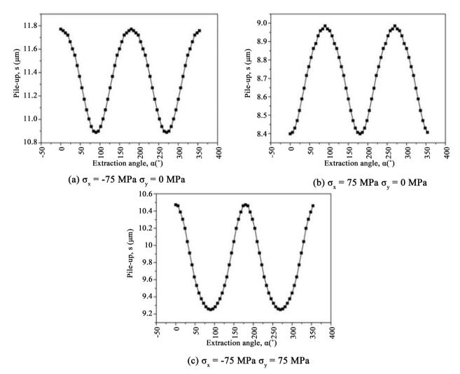
Figure 5. Distribution diagram of maximum pile-up height around the indentation point.
