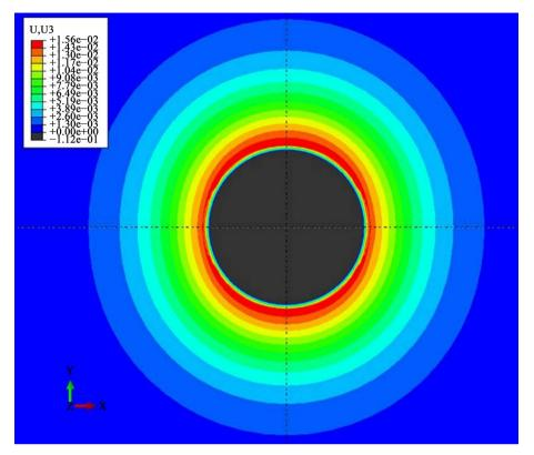
**Figure 3.** Full-field pile-up morphology ( $\sigma_x = -75$  MPa  $\sigma_y = 75$  MPa).
