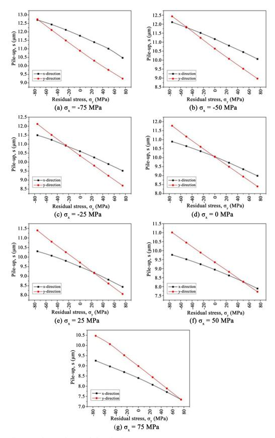
**Figure 4.** Schematic diagram of pile-up height versus  $\sigma_{y}$ .
