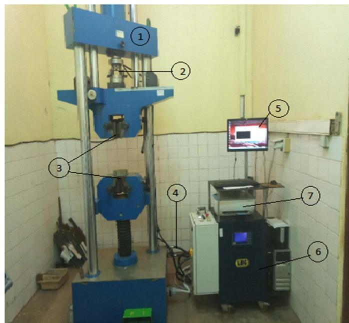
Presentation of the LaboGenie's compression-tension testing device: 1: Universal machine base; 2: Adapted bending test equipment; 3: Tensile-compression testing equipment; 4: Data cable; 5: Data reading interface; 6: Control unit; 7: Printer.
