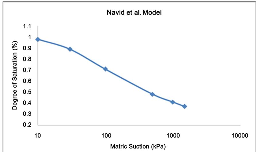
**Figure 1.** Soil-water characteristic curves for soil samples using Navid et al. Model.
