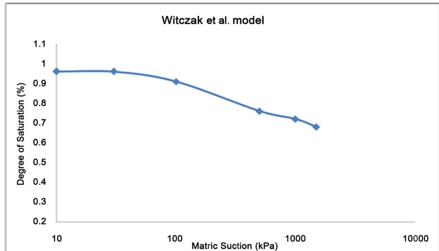
Figure 3. Soil-Water Characteristic Curves for soil sample using Witczak et al. Model.
