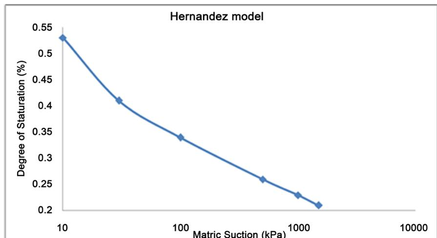
Figure 4. Soil-water characteristic curves for soil samples using Hernandez model.
