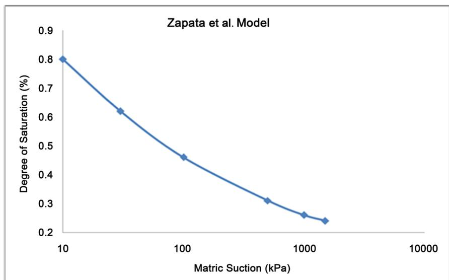
**Figure 2.** Soil-Water Characteristic Curves for soil sample using Zapata et al. Model.
