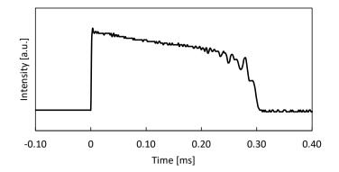
Figure 1. Temporal change of laser pulse strength.
