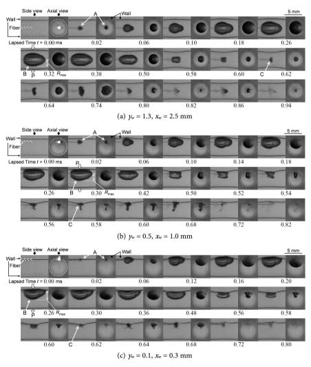
**Figure 4.** Behaviors of a laser-induced bubble and an elastic wall.  $T_w = 16^{\circ}\text{C} - 20^{\circ}\text{C}$ ,  $\beta = 7.3 \text{ mg/L}$ .
