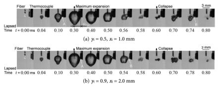
**Figure 6.** Behaviors of a laser-induced bubble near a thermocouple.  $T_w = 20^{\circ}\text{C} - 21^{\circ}\text{C}$ ,  $\beta = 7.7 - 7.6 \text{ mg/L}$ .
