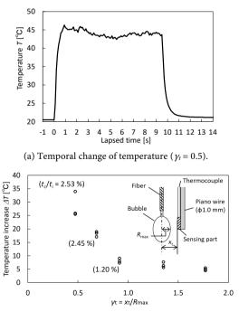
(b) Spatial distribution of temperature increase. *t*: duration of pulsed laser irradiation (10 sec), *t*: total bubble contact time.
