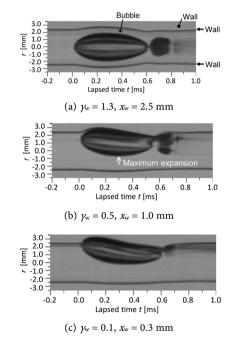
**Figure 5.** Temporal change of a laser-induced bubble and an elastic wall.  $T_w = 16^{\circ}\text{C} - 20^{\circ}\text{C}$ ,  $\beta = 7.3 \text{ mg/L}$ .
