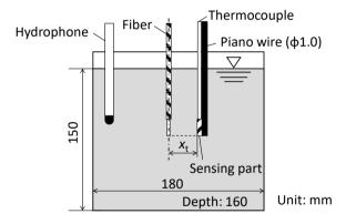
Figure 3. Test section for temperature measurement.
