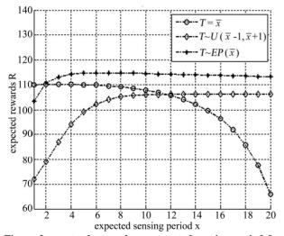
Figure 2. expected rewards vs. expected sensing period for voice traffic.
