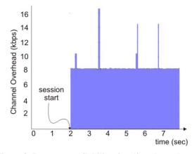
Figure 8. Resource availability signaling channel overhead in the worst case scenario (signaling period: 1 sec.)
