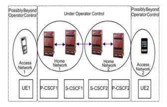
Figure 1. The end-to-end IMS network including access networks
