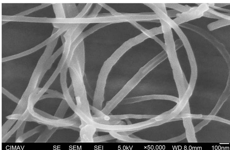
**Figure 2.** High resolution Scanning Electron Microscopy (SEM) micrograph to identify the topographic distribution of MWCNTs (0.05 mg/dl in SRS) applied on a glass coverslip. Magnification  $\times 50,000$ , scale bar 100 nm.
