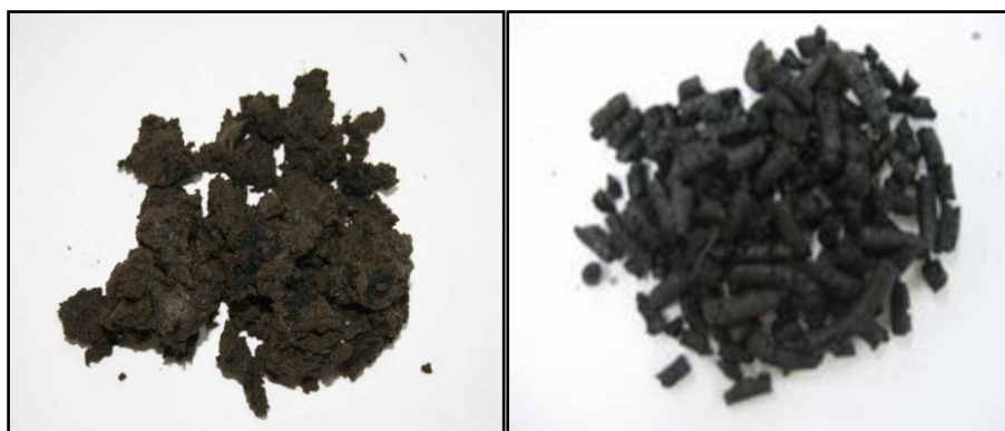
Figure 2. Photography of before and after fry-drying sewage sludge.
