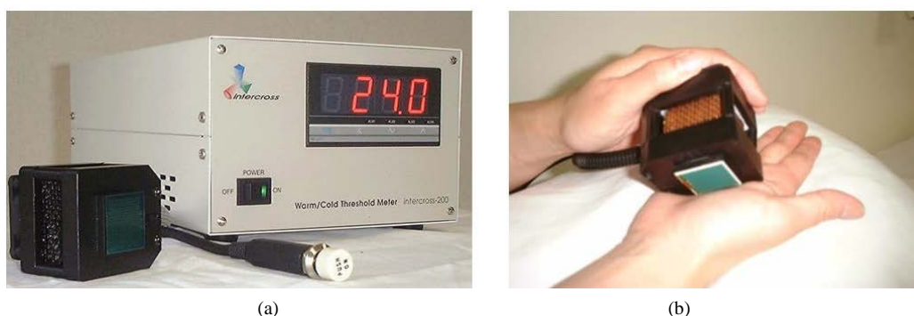
Figure 1. (a) The thermostimulator (Intercross-200, Intercross Co., Tokyo, Japan) comprising a probe, a push-button switch and thermocontroller; (b) Region measurement, on thenar of the non-handedness side.
