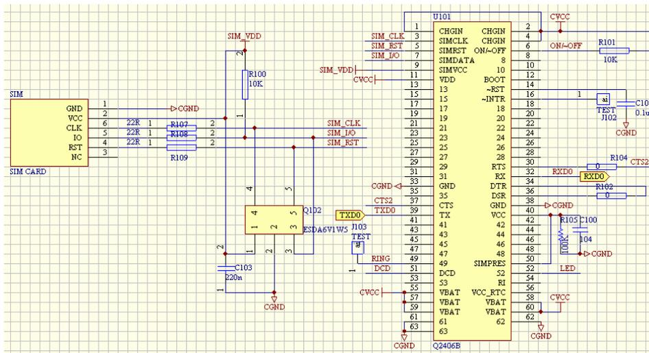
Figure 5. GPRS Module Interface Circuit
