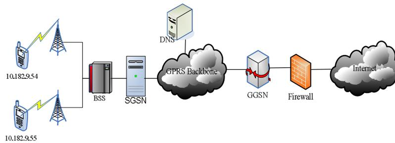
Figure 1. GPRS Principle Structure Diagram
