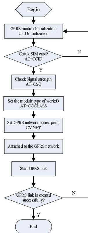
Figure 6. Flowchart of Establish GPRS Links
