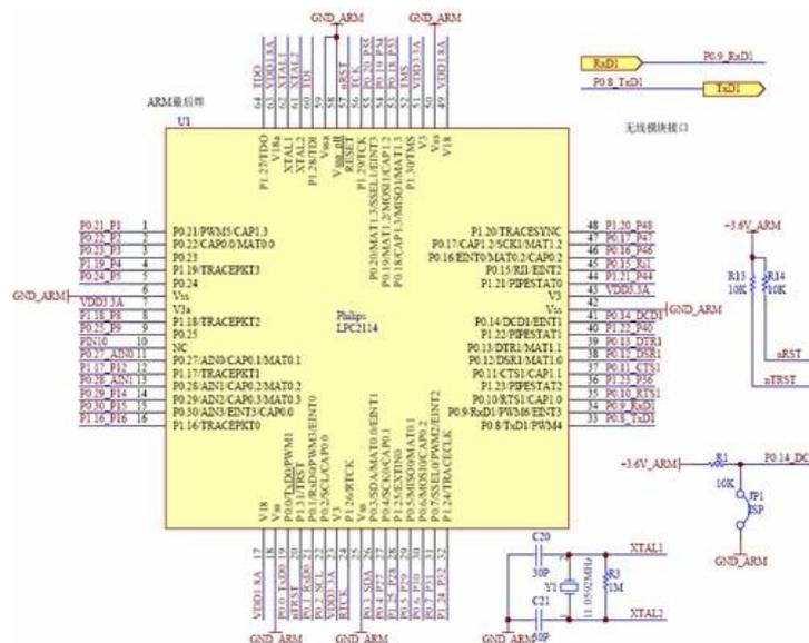
Figure 4. ARM Interface Circuit
