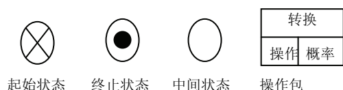
Figure 2. the elements in a state diagram
