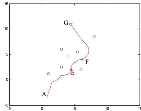
Figure 3. The path planning based on artificial potential field theory
