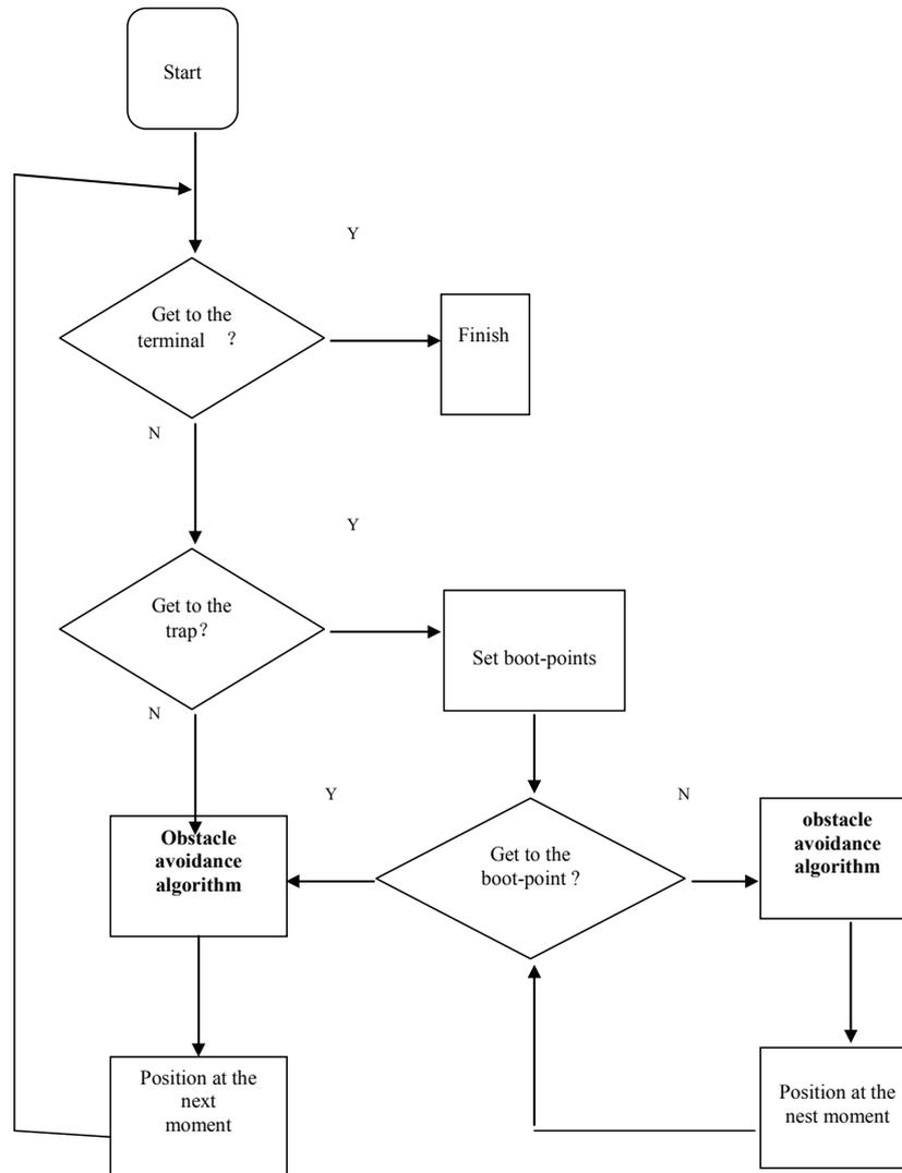
Figure 1. Setting boot-point algorithm
