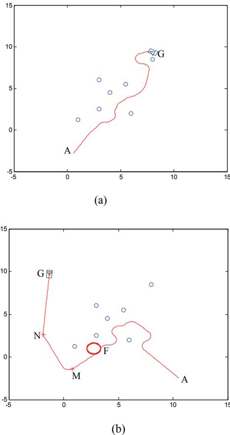
Figure 2. Simulating effects of improved obstacle avoidance algorithm based on the artificial potential field
