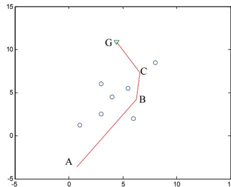
Figure 4. The path planning based on line theory
