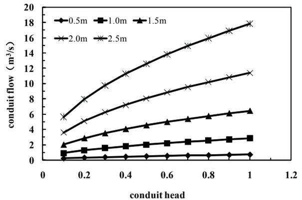
**Figure 3.** Conduit flow corresponding to conduit head and diameter
