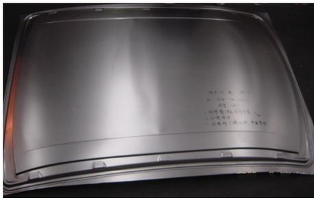
Figure 10. Stamping part of spring-back controlled
