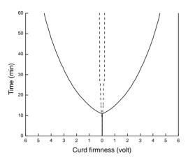
Figure 1. Example of results of curdling dairy cow (continuous line) as opposed to horse (dashed line) as speed tests, coagulation and strength are obtained using the optigraph device.
