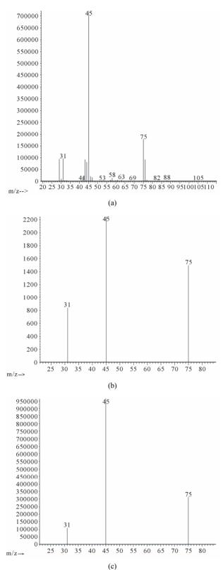
Figure 2. DEG mass spectra obtained from full scan and single ion monitroing (SIM) modes. 2(a) (top) was from full scan detection; 2(b) (middle); and 2(c) (bottom) were from SIM detections.
