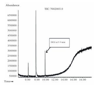
Figure 3. A typical GC-MS chromatogram of DEG with the improved ethanol extraction procedure.
