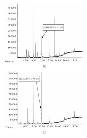
Figure 1. Two typical GC-MS chromatograms of unknown toothpaste spiked with DEG analytes. Figure 1(a) (top) presents an interfering peak just before the DEG peak at retention time 9.9 min and Figure 1(b) (bottom) presents an interfering peak just after the DEG peak at retention time 9.8 min. (Note that DEG peak retention time was shifted after numerous sample analyses).
