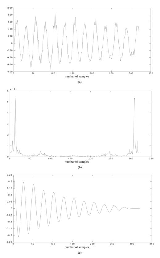
Figure 4. Testing the ACF feature. (a) A speech signal with the fundamental frequency near the first formant; (b) The spectral domain; (c) The ACF.
