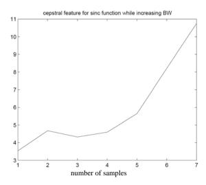
Figure 8. Cepstral feature for the sinc function when increasing BW.
