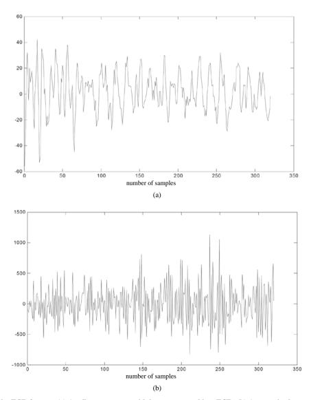
Figure 5. Testing the ZCR feature. (a) A scilence segment with low energy and low ZCR; (b) An unvoiced segment with high ZCR.
