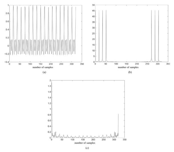
Figure 7. Testing the sinc function for the first category. (a) A sample sinc function with high frequency coefficients; (b) The spectral domain; (c) The cepstral domain, peak to average = 6.
