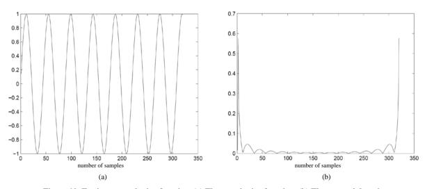
Figure 10. Testing a sample sine function. (a) The sample sine function; (b) The cepstral domain.
