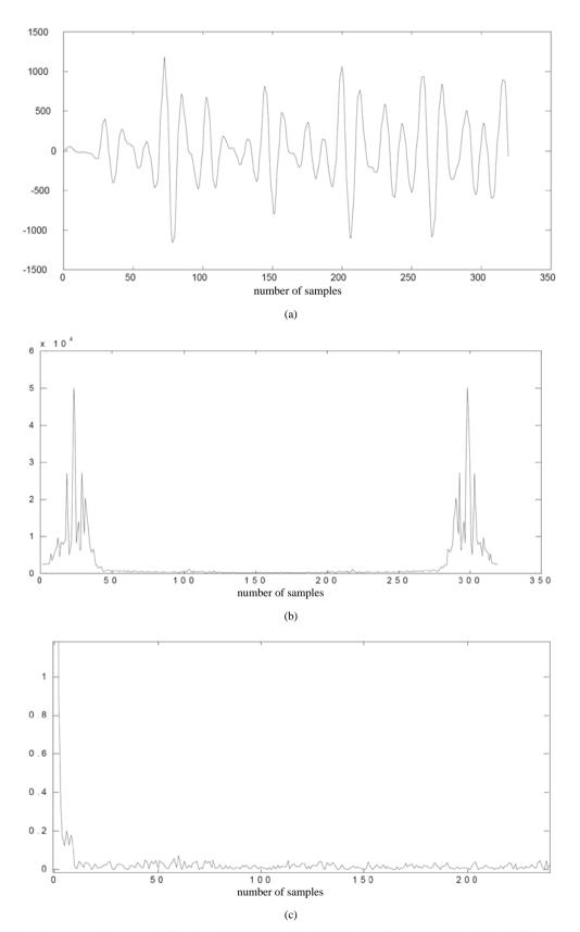
Figure 2. Testing the cepstral feature. (a) The signal with limited bandwidth; (b) The spectral domain; (c) The cepstral domain.
