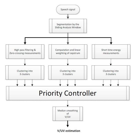
Figure 1. The block diagram of the proposed algorithm.
