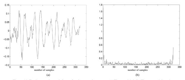
Figure 11. Testing a real speech frame for the second category. (a) The nasal /n/; (b) The cepstral domain.
