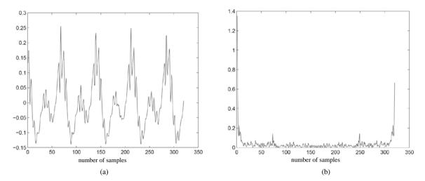
Figure 9. Testing a real speech frame for the first category. (a) The vowel /i:/ as in sheet; (b) The cepstral domain.
