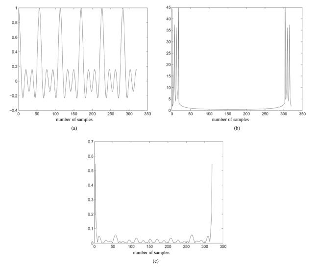
Figure 6. Testing the sinc function for the first category. (a) A sample sinc function with limited bandwidth; (b) The spectral domain; (c) The cepstral domain, peak to average = 3.69.
