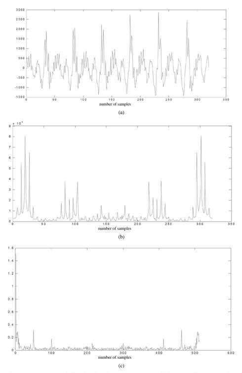
Figure 3. Testing the cepstral feature. (a) The signal with high frequency coefficients; (b) The spectral domain; (c) The cepstral domain.
