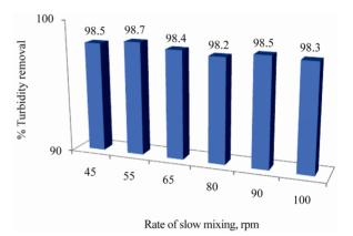
Figure 7. Effect of Rate of slow Mixing on turbidity removal.
