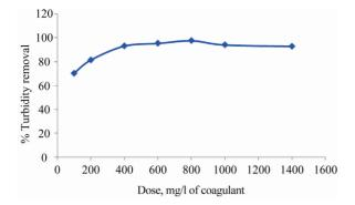
Figure 5. Effect of Coagulant Dose on turbidity removal.
