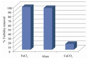
Figure 1. Effect of different coagulants on turbidity removal.
