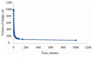
Figure 8. Settling rate of the sludge.
