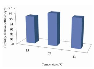
Figure 9. Effect of Temperature on turbidity removal.
