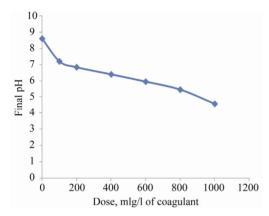
Figure 3. Effect of coagulant dose on solution pH.
