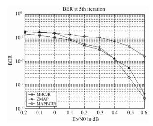
Figure 8. BER comparison between Full-MAP, M-BCJR and Z-MAP turbo decoding at 5<sup>th</sup> iteration.
