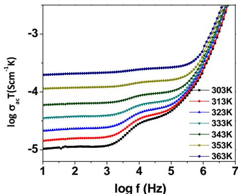
**Figure 6.** Frequency dependence of ac conductivity for  $x = 10$  mol% sample.
