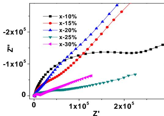
Figure 3. Complex impedance plots of (PbI<sub>2</sub>-CuI-Ag<sub>2</sub>O -V<sub>2</sub>O<sub>5</sub>-B<sub>2</sub>O<sub>3</sub>) glass series at 303K.
