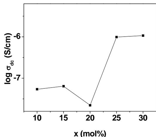
Figure 5. Composition-wise variation of dc conductivity at ambient temperature.
