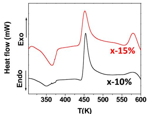
Figure 2. DSC thermogram for  $x = 10$  mol% and 15 mol%.
