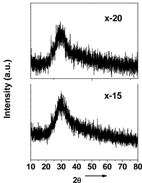
Figure 1. XRD patterns, for  $x = 15$  and 20 mol%.
