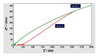
Figure 5. Electrochemical impedance spectroscopy (nyquist Plots) of alumina\_titania coated samples: Al-Ti C (Conventional), Al-Ti N (Nanostructured).
