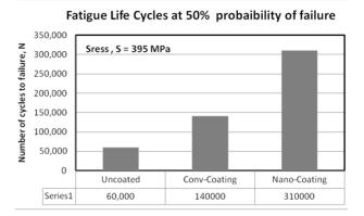
Figure 8. Fatigue life (cycles) for coated and uncoated specimens.
