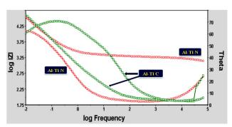
Figure 6. Electrochemical impedance spectroscopy (bode plots) of alumina-titania coated samples: Al-Ti C (Conventional), Al-Ti N (Nanostructured).
