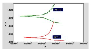
Figure 7. Polarization resistance measurments in NaCl solution.
