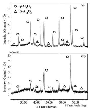
Figure 2. X-ray diffraction of the AT-13 sprayed coatings: (a) conventional coating; (b) nanostructured coating.
