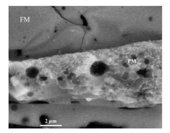
Figure 4. The partially melted region 'PM' consists of  $\alpha$ -Al<sub>2</sub>O<sub>3</sub> (dark) embedded in TiO<sub>2</sub>-rich amorphous phase.
