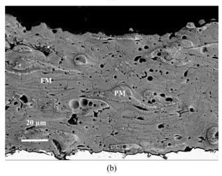
Figure 3. Cross-sectional morphologies of the as-sprayed AT-13 coatings: (a) conventional; (b) nanostructured.
