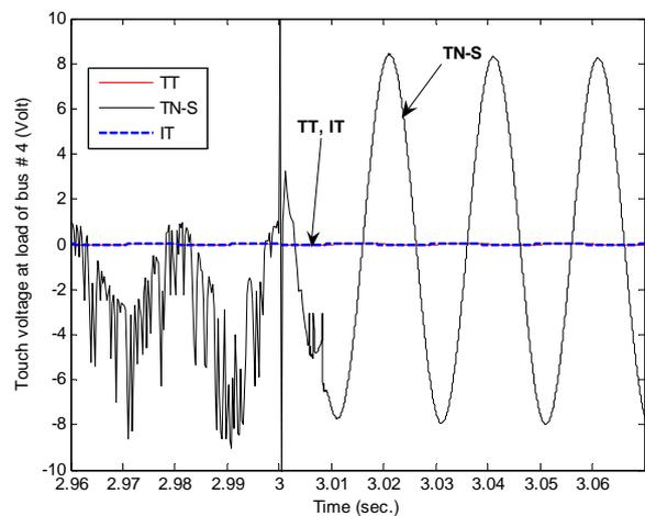
**Figure 11. Touch voltage at consumer of bus # 4.**
