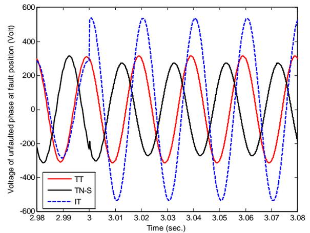
Figure 15. Voltage of healthy phases (at bus # 2).
