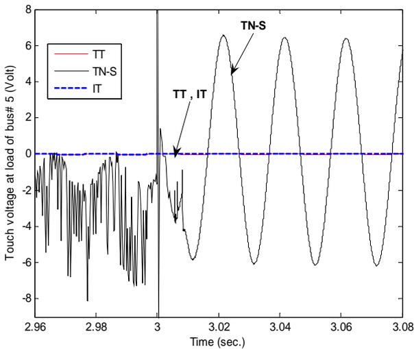
Figure 12. Touch voltage at consumer of bus # 5.
