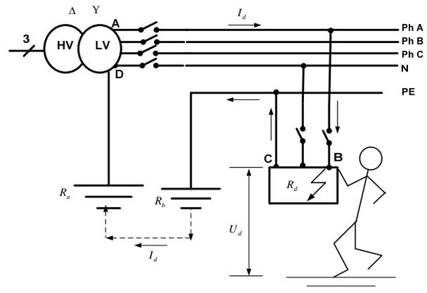
**Figure 5. The fault behavior in the TT earthing system.**
