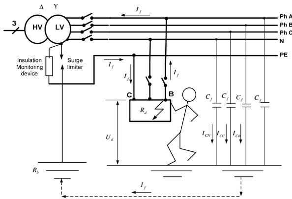
**Figure 6. First insulation fault current in the IT earthing system.**
