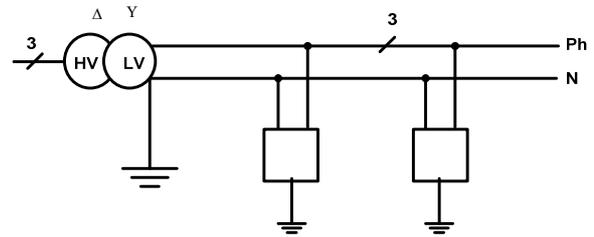
**Figure 1. TT earthing system configuration.**
