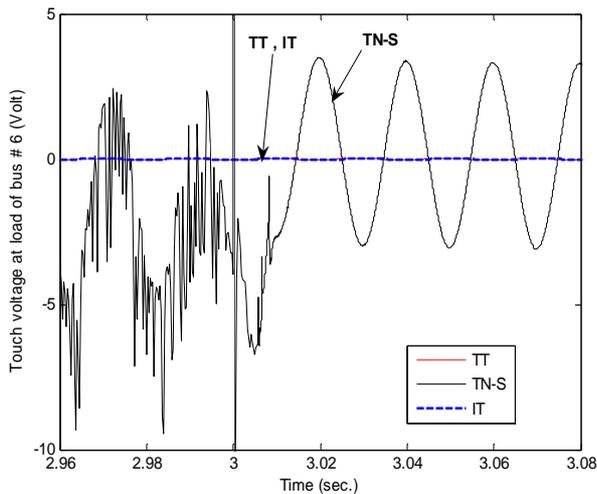
Figure 13. Touch voltage at consumer of bus # 6.
