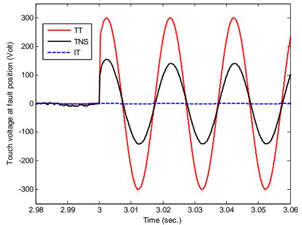
**Figure 10. Touch voltage at consumer of bus # 2 (faulted bus).**
