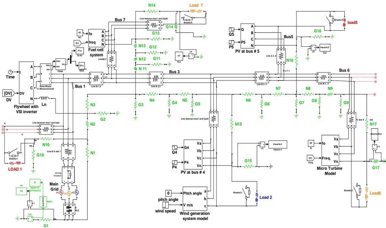
Figure 17. Matlab® /Simulink® Developed model for MG with the earthing system.
