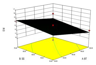
Figure 7. Extrudate moisture (EM) as influenced by screw speed (SS) and barrel temperature (BT).
