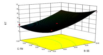
Figure 1. Residence time (RT) of extrudate as influenced by feed moisture content (FM) and screw speed (SS).
