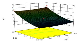
Figure 2. Residence time (RT) of extrudate as influenced by barrel temperature (BT) and screw speed (SS).
