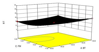
Figure 3. Residence time (RT) of extrudate as influenced by barrel temperature (BT) and feed moisture (FM).
