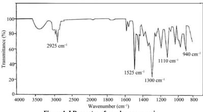
Figure 1. I.R. spectra of novolac epoxy resin.
