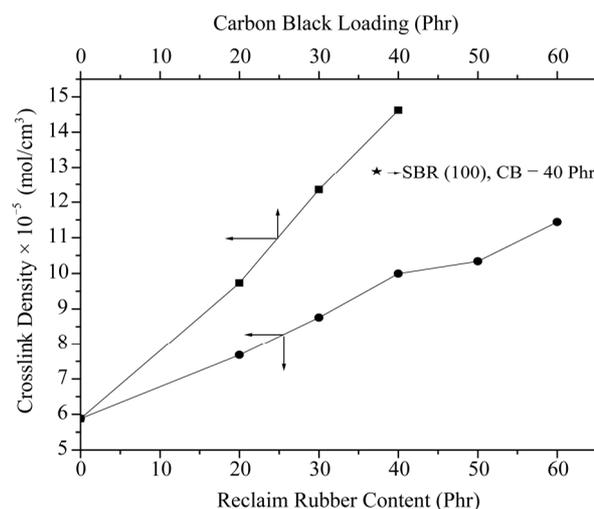
**Figure 2.** Crosslink density of SBR/RR blend system as a function of reclaim rubber content and carbon black loading.
