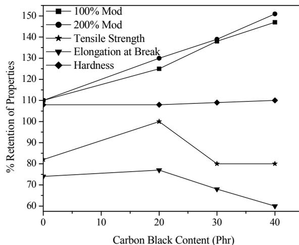
Figure 8. Effect of carbon black loading on % Retention of properties after 72 h aged SBR/RR (80/20) blend system.
