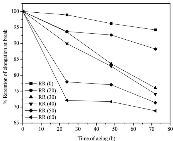
Figure 6. Effect of reclaim rubber content on % retention of Elongation at Break.
