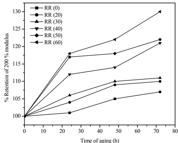
**Figure 4.** Effect of reclaim rubber content on % retention of 200% Modulus.
