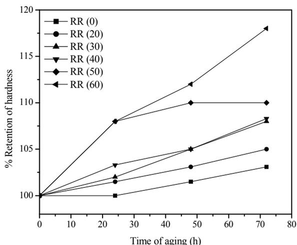
Figure 7. Effect of reclaim rubber content on % retention of Hardness.
