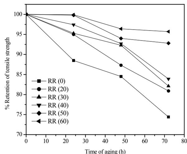
**Figure 5.** Effect of reclaim rubber content on % retention of Tensile Strength.
