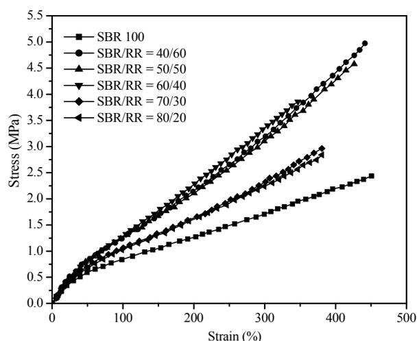
**Figure 1.** Stress – Strain behavior of SBR/RR blend system.
