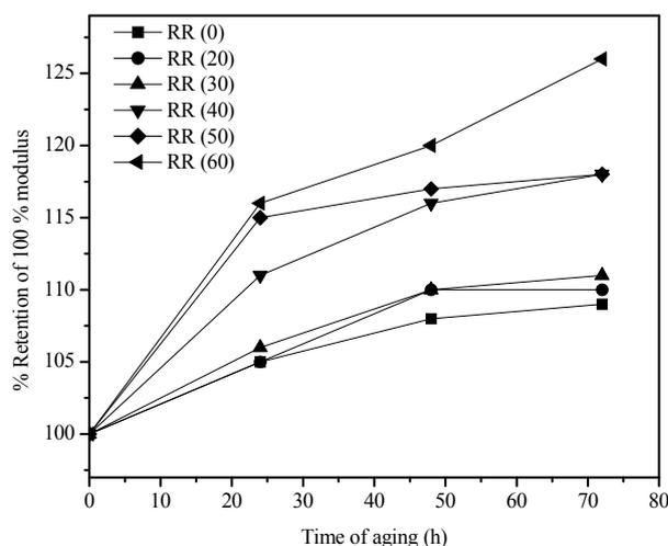
**Figure 3.** Effect of reclaim rubber content on % retention of 100% Modulus.
