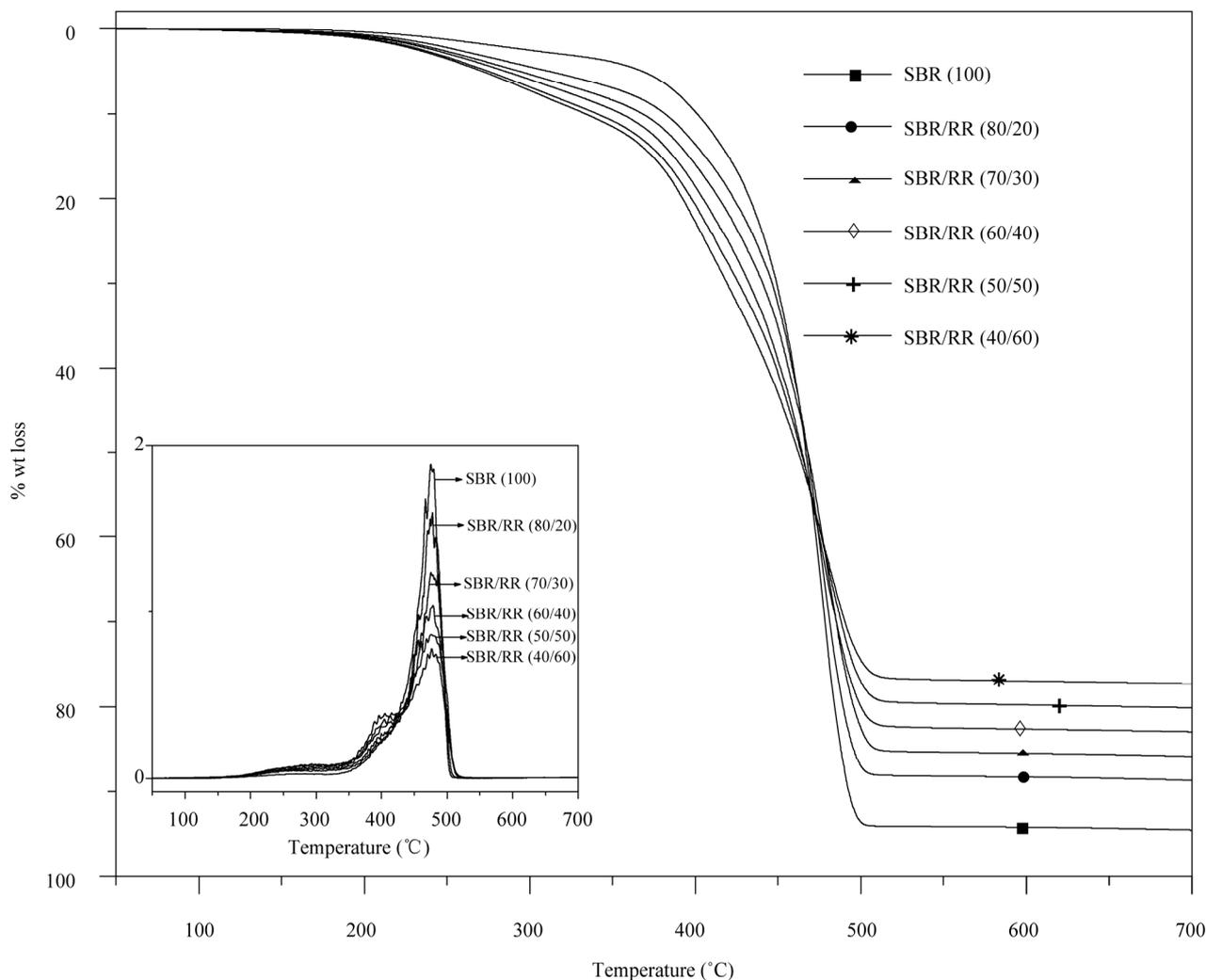
Figure 9. Thermogravimetric analysis of SBR/RR Vulcanizates.
