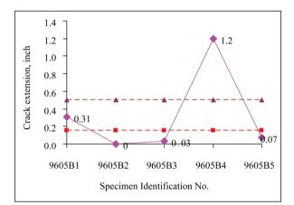
Figure 1. Crack wedge length of bare Al.
