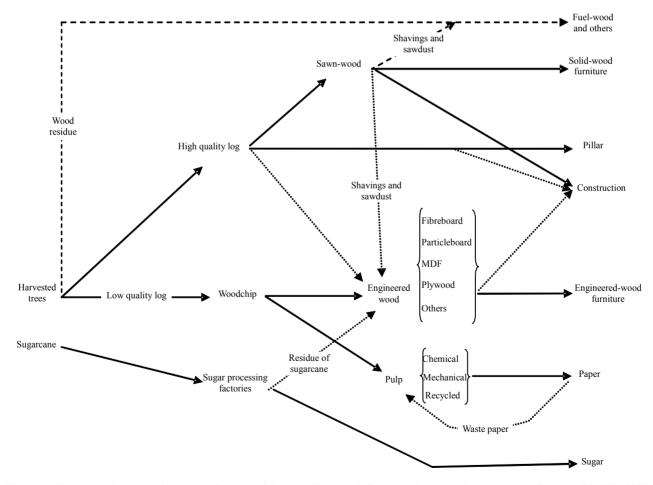
Figure 1. Inputs and outputs for manufacture of intermediate and final wood-processing products. Source: ICARD [34], ICARD [35], Barney [29], Nguyen *et al.* [35], Nguyen *et al.* [36], Lamb *et al.* [37] and Phan *et al.* [6].
