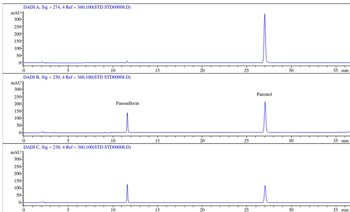
**Figure 1.** HPLC profiles of paeoniflorin and paeonol standards at three detection wavelengths. Chromatograms are shown for detection at 274 nm (top panel), 230 nm (middle), and 238 nm (bottom). Paeoniflorin was detected at 11.6 min; paeonol, at 27 min. Based on these profiles, 230 nm was selected as the detection wavelength for subsequent qualitative and quantitative HPLC analysis.
