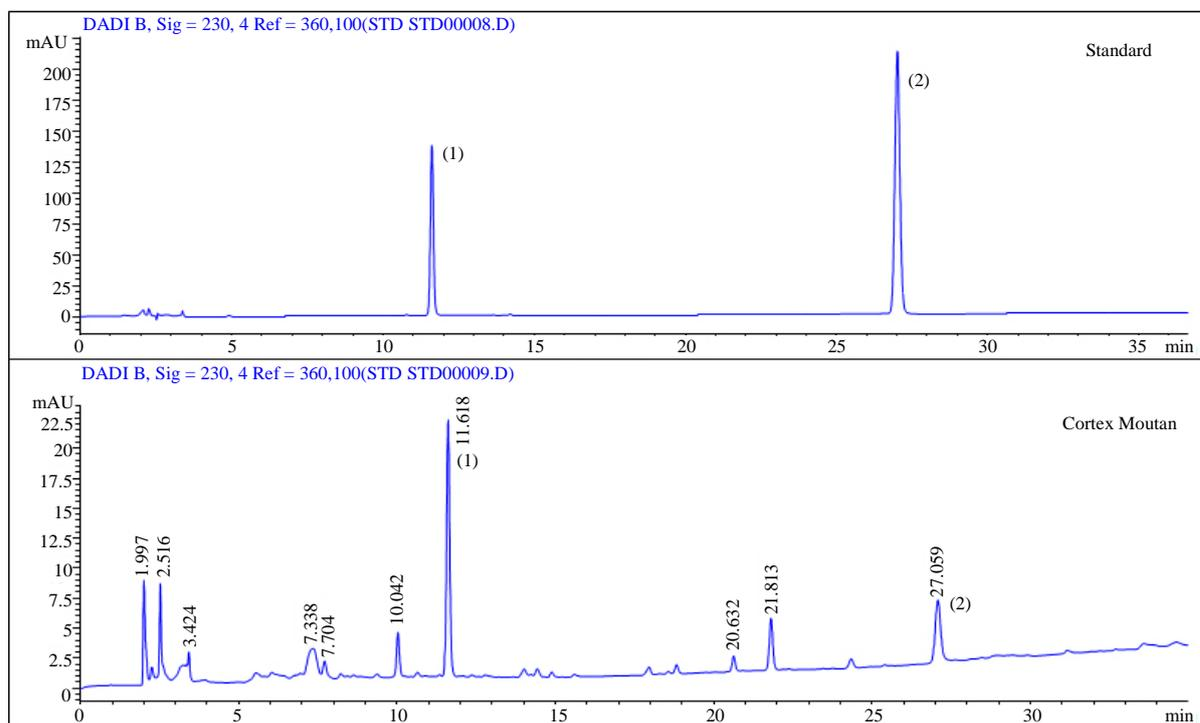
**Figure 2.** HPLC-UV analysis of Cortex Moutan. Standards containing the target analytes, paeoniflorin (peak 1; retention time, 11.6 min) and paeonol (peak 2; retention time, 27 min), were used to calibrate the HPLC instrument. Both analytes were among the main compounds detected in the Cortex Moutan sample.
